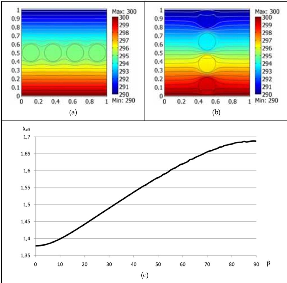
Fig. 2. (a) Horizontal alignment,  $\lambda_{eff}=1,37$  (b) Vertical alignment  $\lambda_{eff}=1,68$  (c) Relation between effective thermal conductivity  $\lambda_{eff}$  and the angle  $\beta$  of rotation of four fibres aligned. The conductivity of matrix  $\lambda_M=2$ , fibres conductivity  $\lambda_F=0.1$ . Fibres radius  $R=0.1$
